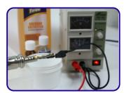
Now the electrolyte has to be prepared: mix about 0,5 - 1% of the gelling agent (Tifoo gelling agent) with the required amount of electrolyte solution.
