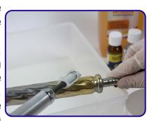
Make sure that the power supply indicates a peak of current. If this is not the case, check again if everything is properly connected and if the swab is saturated with the electrolyte solution. Immerse then the swab at regular intervals into the reservoir of the gold electrolyte. After a short time a considerable part of the surface is already completely gold plated.
