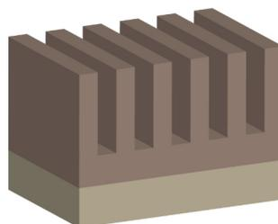
This means that the anodic coating is anchored directly in the original aluminium and can no longer be removed mechanically. These pores are able to absorb liquids, e. g. dyes, after the anodization process.
