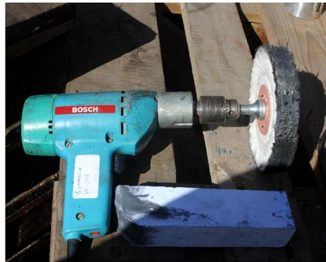
You proceed in the following way: fasten the molleton wheel to the corresponding drill and rub some polishing paste onto the wheel (while this wheel is turning) and rub a bit of the paste also over the object. Then, you polish the object as shown on the following picture:
