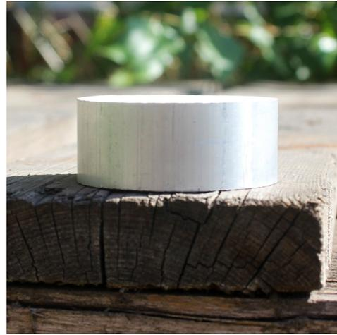
The surface, dull but otherwise in a good condition, was polished to a high sheen with a molleton wheel, which is an attachment available for conventional drills, by using a polishing paste.
