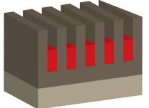
After a dye has been embedded into these pores, you can again close the oxide layer by the so-called sealing. This means that aluminium oxide reacts with water and crystallizes to hydrate alumina (Al2O3 x H2O) which clogs the pores.
