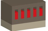
The dye is thereby are permanently bound to the aluminium and cannot be scraped off or flake like varnishes for example. It is of course also possible to not embed any dye or to seal the oxide layer directly after anodizing; then, the work piece keeps its silvery grey colour yet is nevertheless protected against corrosion.
