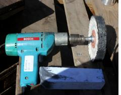
You proceed in the following way: fasten the molleton wheel to the corresponding drill and rub some polishing paste onto the wheel (while this wheel is turning) and rub a bit of the paste also over the object. Then, you polish the object as shown on the following picture:
