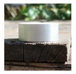
The surface, dull but otherwise in a good condition, was polished to a high sheen with a molleton wheel, which is an attachment available for conventional drills, by using a polishing paste.
